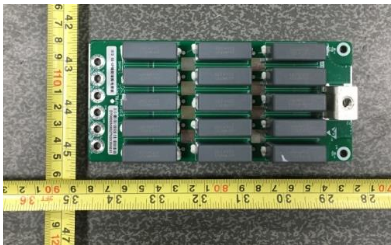
Figure 8 Front of filter board
